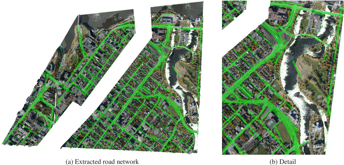
Figure 5. Screenshot of the road network for the entire point cloud that contains 166 million points and covers 3 \times 3\text{km} . Our approach successfully extracts roads with varying width, large curved sections and bridges with limited false positives and missed detections.
