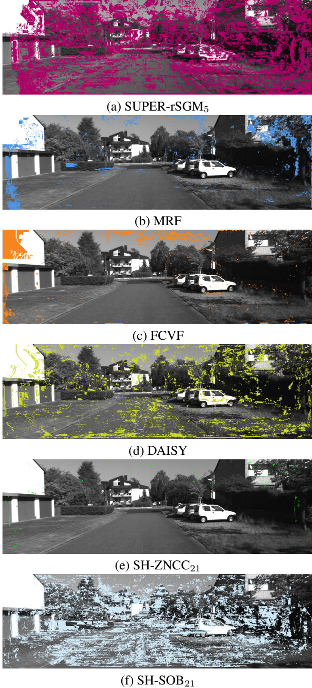
Figure 2: Each subfigure highlights the pixels that selected the corresponding disparity of each matcher. The top six (out of eight) matchers are shown. SUPER-rSGM 5 and SH-SOB 21 dominated the disparity selection for this stereo pair.
