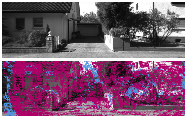
Figure 1: An input frame and a visualization showing pixels colored according to the matcher that was selected for them by the classifiers. Pixels from only two matchers are shown for clarity.
