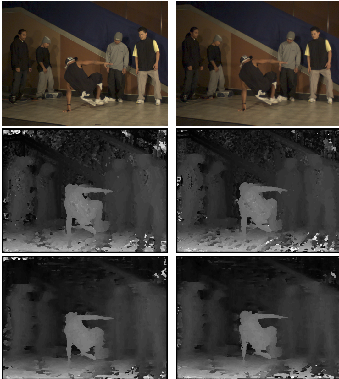
Figure 4. Results for cameras 3 and 4. The top row is the color reference images. The second row is the initialization (from plane sweep[3]), the next is the result after nine iterations.
