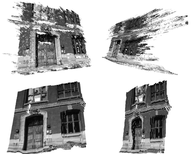
Figure 7. Screenshots of results on our sequence. Top: point cloud reconstructed from input fused depth maps. Bottom: point cloud of surface voxels after diffusion.
