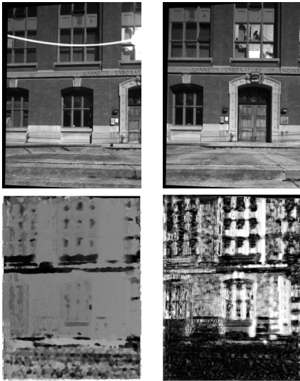
Figure 6. Two of the input images from our sequence and the fused depth and confidence maps for the image on the left. Notice the CCD blooming in the top left image, which appears curved after radial undistortion. Depth maps contain errors due to lack of texture, reflections on the windows and miscalibration. Fortunately, most of the depth errors are associated with low confidence values.
