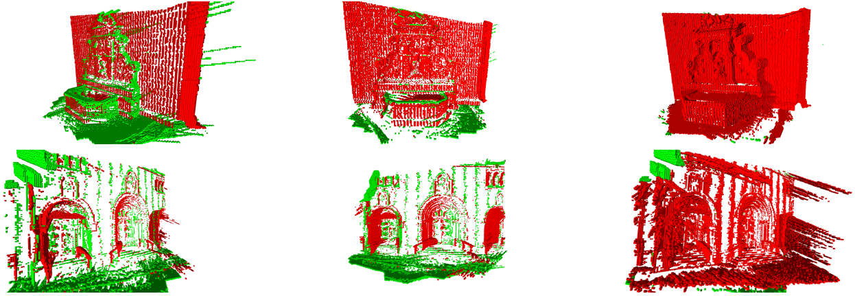
Figure 5. Screenshots of difference grids for both datasets. False positives of occupancy are colored red, missed detections are colored green and voxels in agreement with the ground truth are left blank. Each screenshot is from a different model using different values for \theta , resulting in bias for one type of error over the other.
