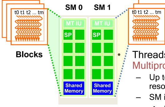
Threads are assigned to Streaming Multiprocessors in block granularity
