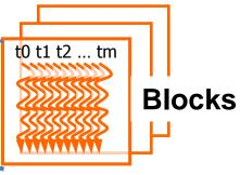
Threads are assigned to Streaming Multiprocessors in block granularity
