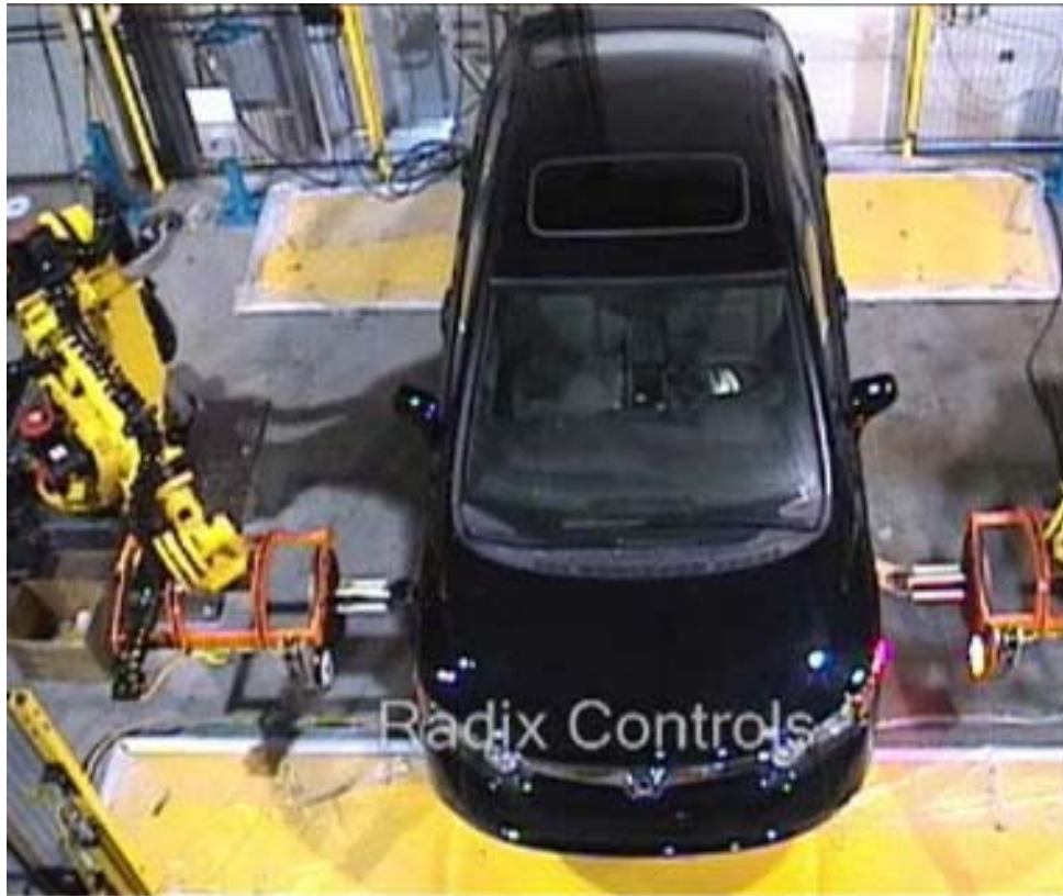
Vision-guided robots position nut runners on wheels
